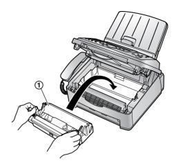
**12** Close the front cover (①) by pushing down on both sides, until locked.
